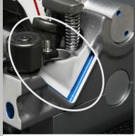
With the solenoid activated, engine oil passes through the Rocker Shaft, and then to the bottom of the Control Valve moving the control valve to index with the high pressure passage in the Exhaust Rocker.
