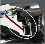
The oil passes through the Control Valve and extends the Actuator Piston to its pre-determined length. The control valve ball check prevents the oil from escaping, locking the actuator piston.
