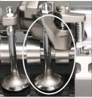
Braking Cam motion is transferred to the Exhaust Valve via the Brake Rocker to the Exhaust Rocker, by interfacing with the extended Actuator Piston.
