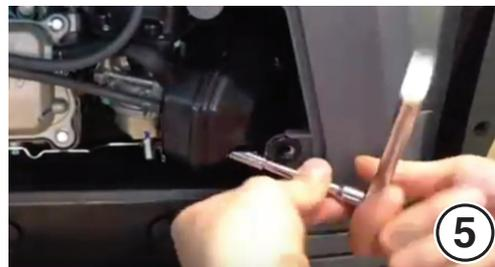
6. Remove the clamp on the vapor tube and set it aside. Remove the vapor tube and the crankcase breather.
