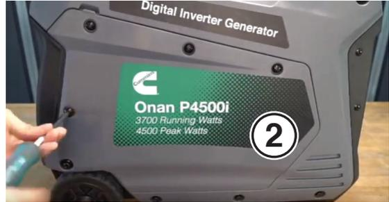
3. Remove the control panel by removing the 4 screws on the face and the two screws on each side. Let the control panel hang loose.
